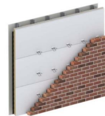
Brick veneer: 1" air gap
