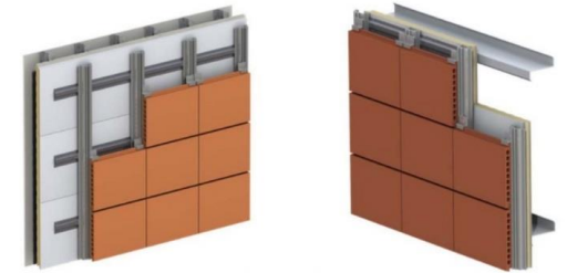
Terra-cotta tile: Minimum continuous \frac{3}{8} " air gap
